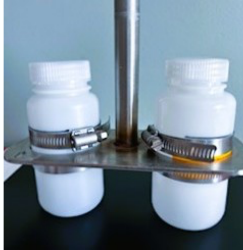
Figure Ap3-2. Sample bottles are placed in the sampling plate with bottom clamps in place. The bottle caps are then removed, and the sampling plate is lowered by the handle to retrieve a duplicate sample.
