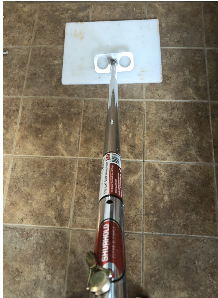
Figure Ap3-3. The extendable aluminum rod is used to lower the sampling plate with the attached bottles into the surface waters at the test site. A loop on the handle allows for an extra line to lower the unit from greater heights as needed.
