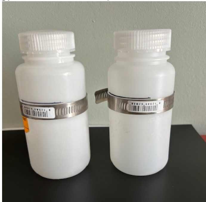
Figure Ap3-1. Two HDPE, 250 mL sample bottles with sterile pipe clamps in place prepared for field sampling prior to being placed in a cooler with ice packs.
